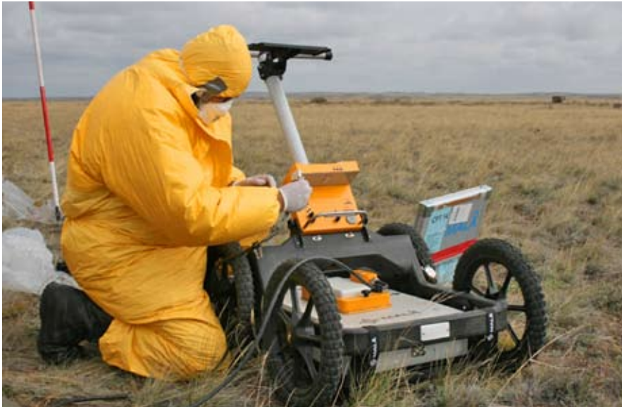
The ground penetrating radar is prepared for use during the inspection period.
