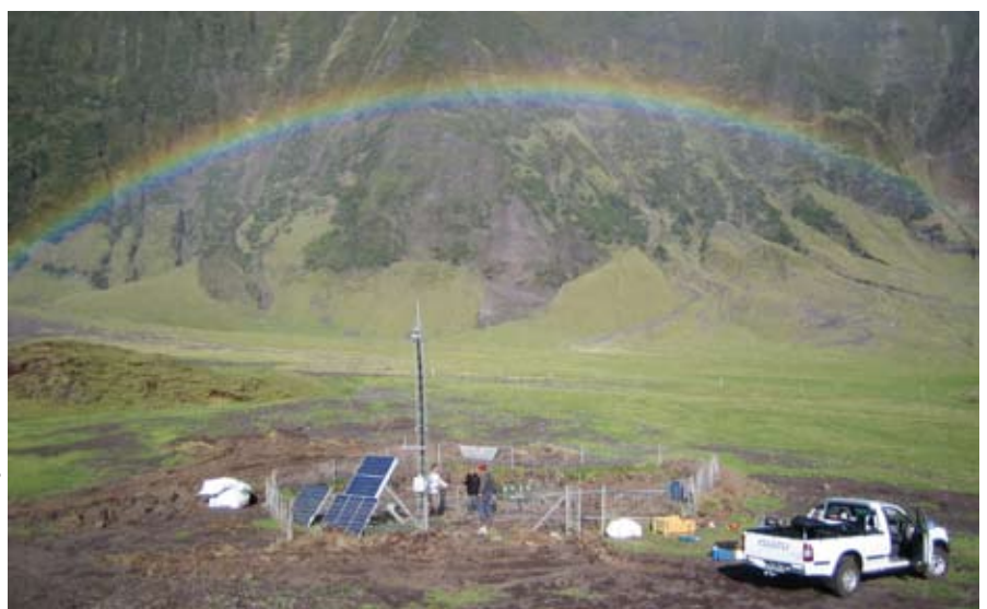
An infrasound station used by the CTBTO to detect very low frequency sound waves produced by natural and man-made events.
