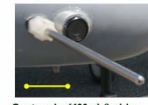
Gust probe (400 g) & video camera (280 g) → turbulence & cloud targeting
