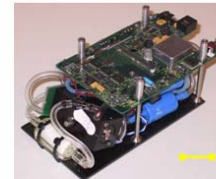
Condensation Particle Counter (870 g) → N_{CPC}; D_p > 10 \text{ nm}
