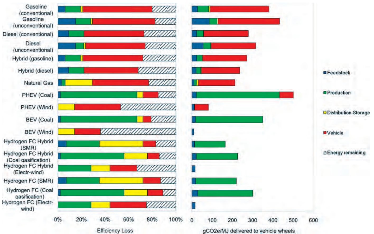
Figure 9.30 | Relative amount of energy required for different supply chains (the shaded area corresponds to the energy remaining at the wheel) and well-to-wheel GHG emission for various powertrain/fuel combinations. Source: based on Creutzig et al., 2011a.
