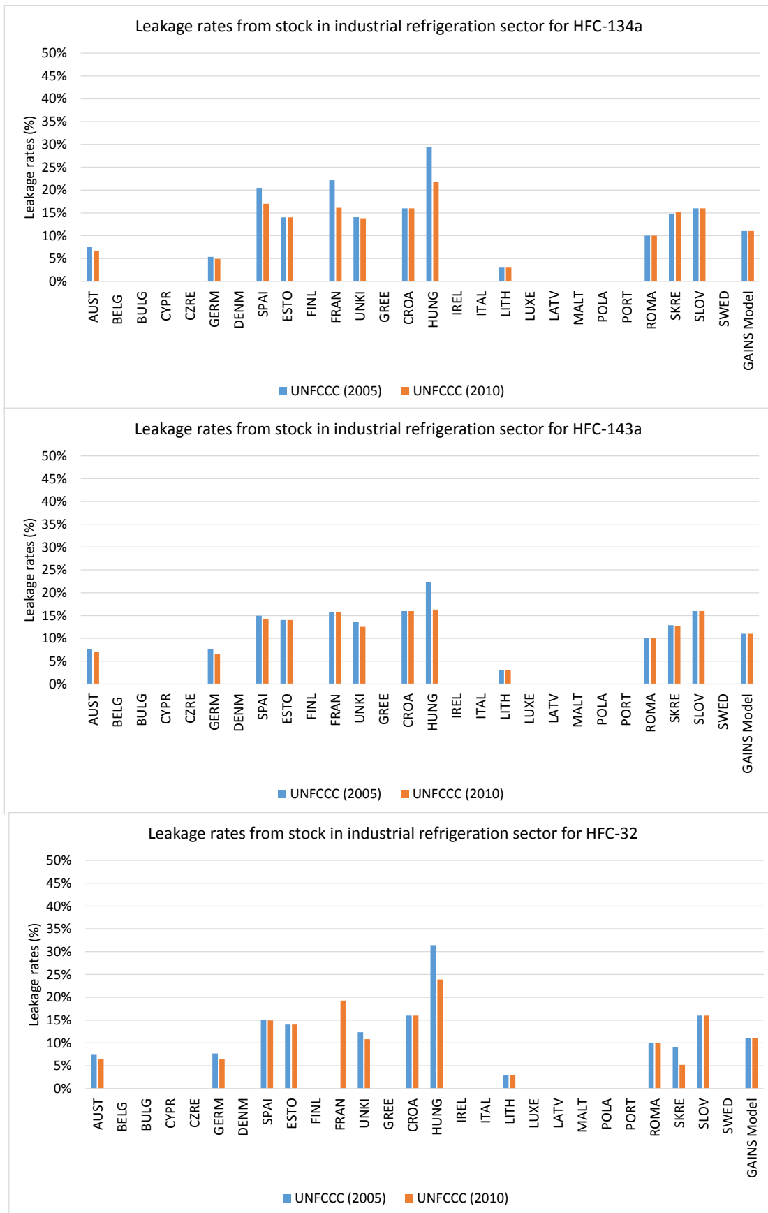
Figure 7: Leakage rates from stock in industrial refrigeration in years 2005 and 2010 for different HFCs as reported to UNFCCC (2015) and assumption adopted in GAINS
