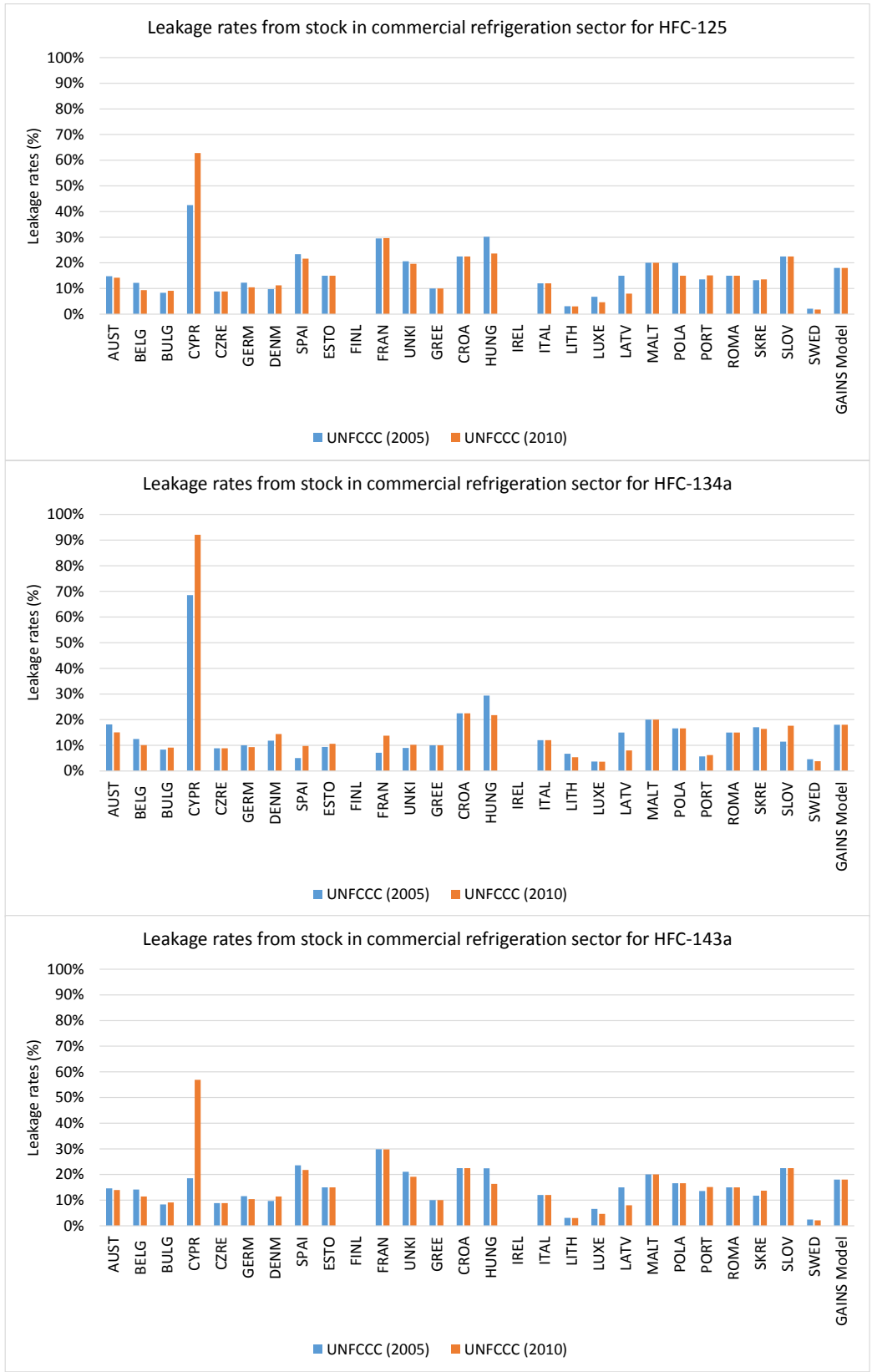
Figure 6: Leakage rates from stock in commercial refrigeration in years 2005 and 2010 for different HFCs as reported to UNFCCC (2015) and assumption adopted in GAINS.
